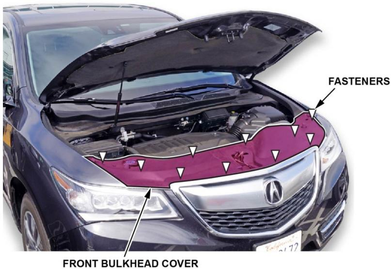
2. Remove the 10 strikers from the bulkhead cover, and the 10 latches from the bulkhead and grille. Do not mix the old latches and strikers with the new parts.
